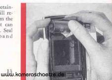
At this time, remove the empty spool and put it in the take-up chamber so your camera will be ready for the next roll of film.
